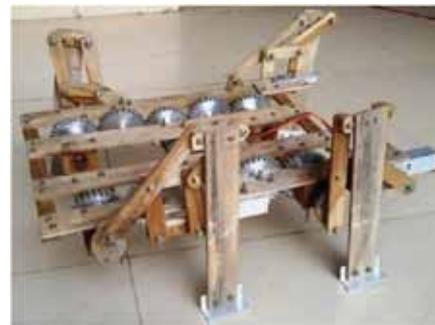
Fig. 2: Prototype of Biologically inspired four legged robotic vehicle
