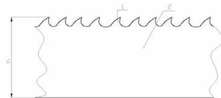
Fig. 3: A bionic cutting band saw
