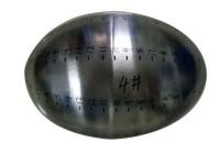
Geometry of the egg-shaped pressure hull
