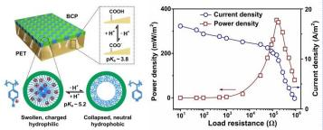
We first develop a proof-of-concept asymmetric bipolar heterogeneous membrane system with ultrahigh ion rectification. The system can achieve a power density approximately 0.35 W/m<sup>2</sup> by mixing river water and sea water, which outperforms many commercial ion exchange membranes.
