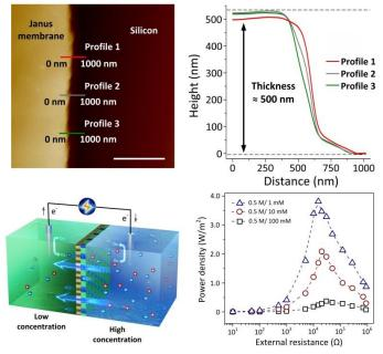
To expand to new avenues and stay economically attractive, membrane development must constantly strive for higher permeability and seek new and better selectivity. Next, we developed a block copolymer based ultrathin Janus membrane with excellent anion selectivity. The sub-micrometer scale thickness ( $\approx$  500 nm) of the system provides very low ion resistance and high permeability,
