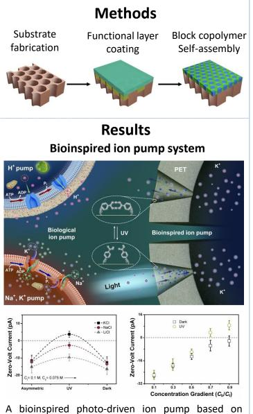
A bioinspired photo-driven ion pump based on single PET conical nanochannels is developed. The pumping process behaving as an inversion of zerovolt current can be realized by applying UV irradiation from the large opening. Enhanced electrostatic interaction between the ions and the charged groups on the inner wall is the key reason.
