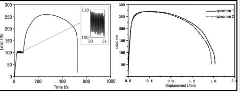
Fig. 3. Tensile and fatigue tests.
