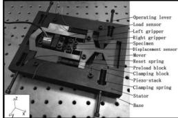
Fig. 1. Structure of the device.
