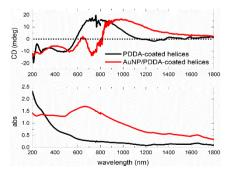
After Au functionalization, the spectral wavelength red-shifted by ~200 nm, with a sharp peak at ~700 nm.
