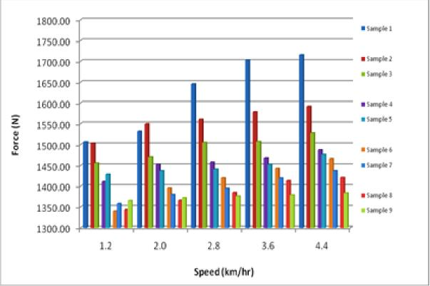
Fig. 3: Effects of Bionic Density on Soil Resistance
